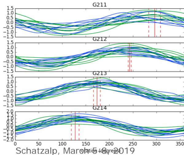
Cross-correlation coefficient as a function of the rotation of the geophone for different borehole levels.
