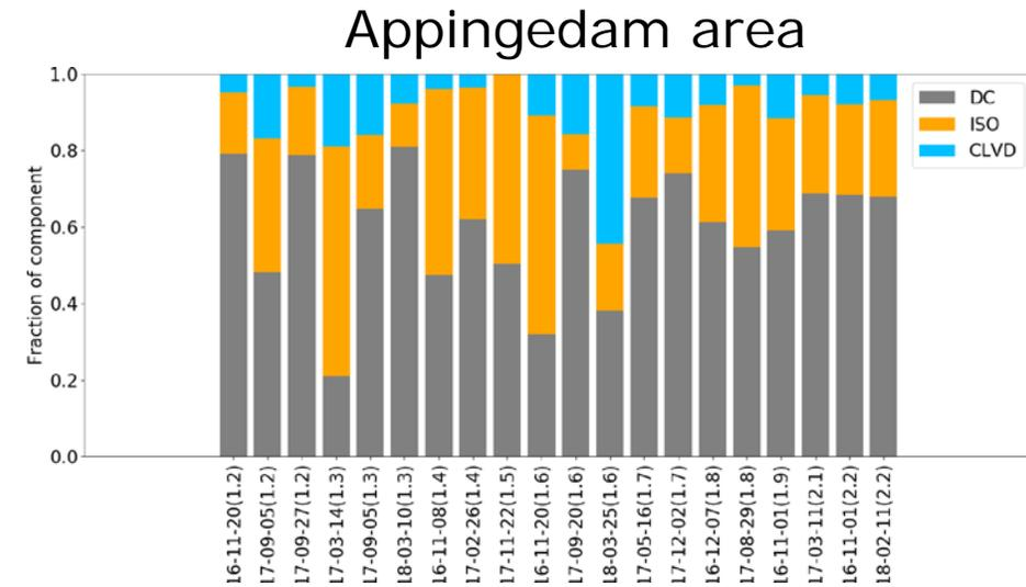
Contribution of Double Couple (DC), Isotrope (ISO) and Compensated Linear Vector Dipole (CLVD) components to the Moment Tensor solutions.
