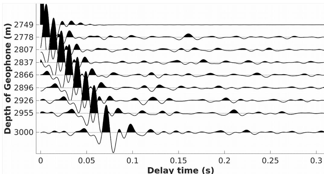
**Fig. 1** Vertical component train noise deconvolutions with signal from the top geophone (Jul-Dec 2015).
