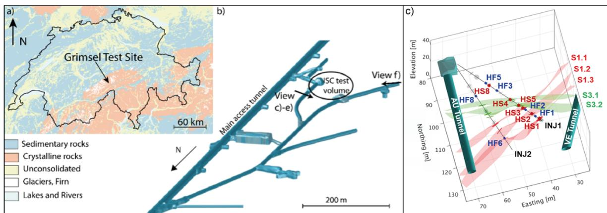
**Fig. 1** Location of the GTS in Switzerland indicated in the geological map (a), and location of the test volume within the GTS (b). The injection intervals are marked together with the target shear zones (c).
