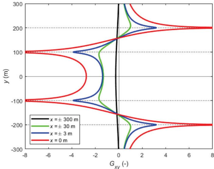
Scaled shear stresses  $G_{xy} = \sigma_{xy}/C$  at constant horizontal distance  $x$  from the fault.
