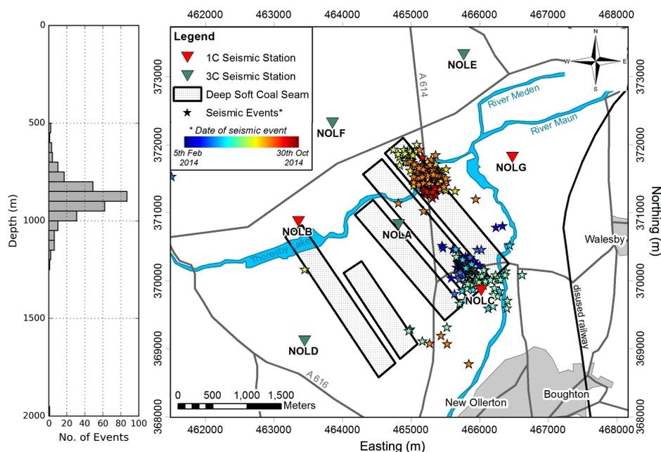
**Fig. 1** Left – Depth distribution of seismic events at New Ollerton, UK. Right - Location of seismic network (inverted triangles), recorded seismic events (stars) and coal seam panels (black rectangles). Seismic events have been coloured coded to show temporal distribution. Position and depth distribution show a strong correlation with the excavated coal panels.
