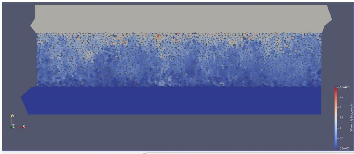
**Fig. 1** Screenshot of a model with 2500 angular grains. Magnitude of the velocity of the grains with imposed shear velocity, simulated with the code MELODY.
