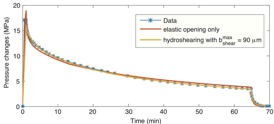
**Fig. 1** Comparison of elastic opening only model (red line) and hydroshearing model with 90  $\mu\text{m}$  maximum aperture (yellow line) with data from Fenton Hill, Test 1 (blue line).
