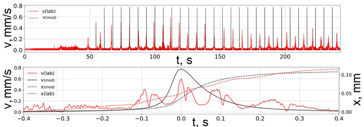
**Fig. 1** Time dependence of block velocity and slip. Laboratory data and result of numerical modeling.
