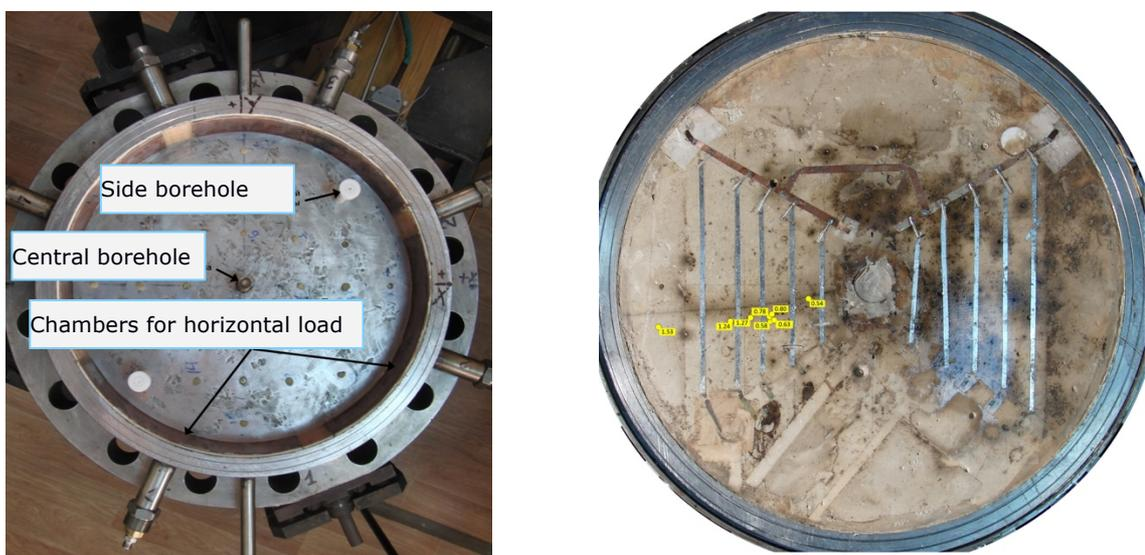
**Fig. 1.** Left: inside view of the laboratory setup; right: the fractured sample, yellow marks show positions of the acoustic emission sources, strips were used to measure the fracture propagation rate.
