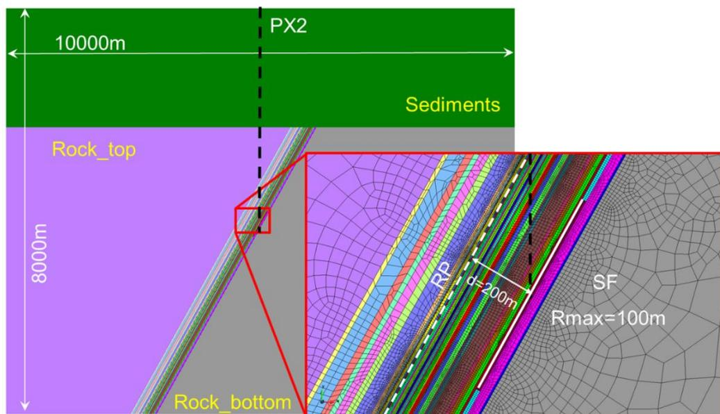
**Fig. 1** 2D vertical domain for poroelastic hydromechanical modelling of the first stimulation in the PX2 well. RP denotes the supposed rupture plane where micro-seismicity has been observed with assumed hydromechanical properties of a fault core zone, water is injected into the source fault SF within the open borehole section of PX2. The hydromechanical parameters of the different fault sections are derived from well logging data.
