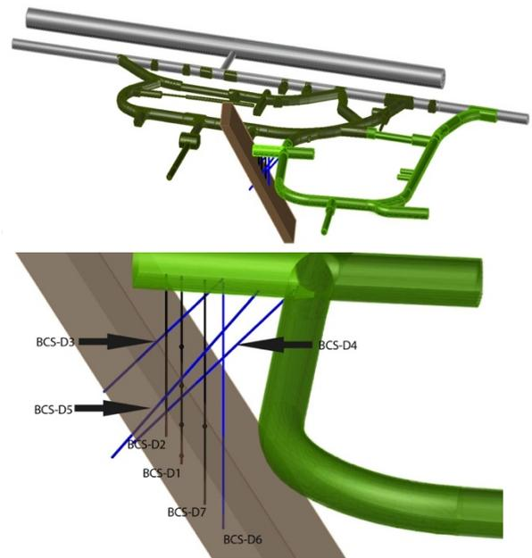
**Figure 1** (top) The Mont Terri Underground laboratory and the fault zone (brown). Niche 8, hosting the CS-D experiment, is in yellow-green. (bottom) Position of the boreholes for injection (BCS-D1), SIMFIP (BCS-D7), fluid monitoring (BCS-D3), and geophysical monitoring (BCS-D3-6).
