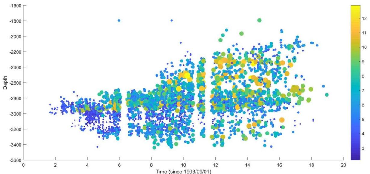
**Figure 1: Time evolution (in day) of the source radius as a function of the depth during the 1993 stimulation of GPK1 (Soultz-sous-Forêts). The colorbar corresponds to the size of the radius in meter.**
