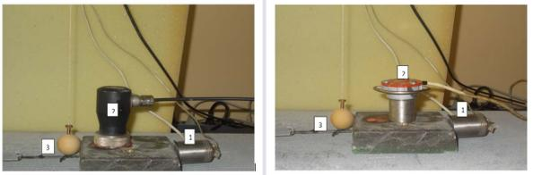
•Seismic vibrator (1) is attached to the sliding plate to which 2.5 v voltage is applied. Registration of the acoustic signal is produced using piezo sensor (2). Calibration of the acoustic signal is produced using pendulum (3).
