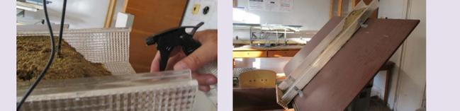
Landslide modelling experiment: (i) by dry sand critical slip angle is approximately 26° degree; (ii) By moderate saturated sand critical slip angle is approximately 60° degree
