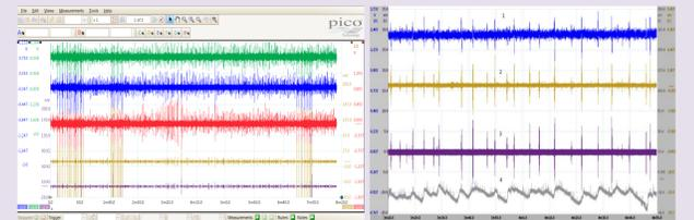
The figure shows recording of the acceleration and acoustic emission on the 8 channel picoscope. In the figure the signals with large amplitude present recordings the pendulum collision on the bottom plate. A series of experiments and data processing is being done on the presented experimental setup.
