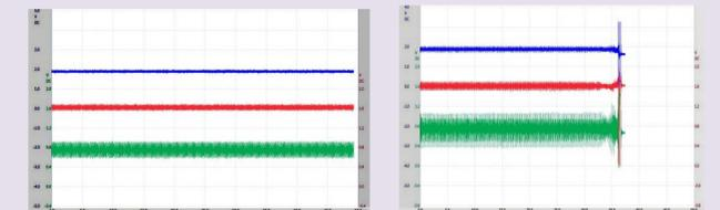
Recordings of the accelerometer: (left) seismic vibrator is placed on the rear surface of the fixed plate, (right) the seismic vibrator is placed on the upper surface of the fixed plate.
