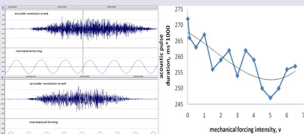
•A single acoustic emission pulse (upper channel) and mechanical forcing (lower channel) on the expanded part of recording shown in Figure. In both cases vibrator was powered by the voltage 4 V: (upper) normal forcing, (down) tangential forcing.
