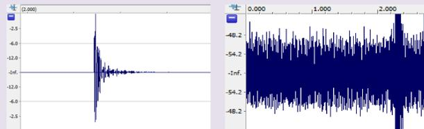
(left) expanded record of acoustic signal generated during clash of 1 cm deviated pendulum using seismic sensor; (right) expanded record acoustic signal on piezo sensor under action of seismic vibrator to which 2.5 v voltage is applied with accompanying noise; (y - axis acoustic signal intensity in dB, x - axis time in ms).
