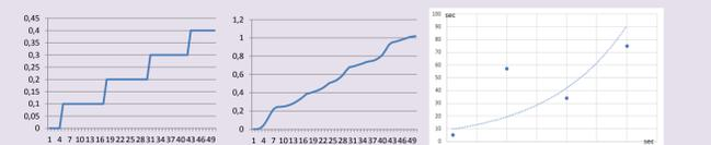
•Numerical simulation of displacement (ordinate) versus time (abscissa) for one block, •the same calculations carried out for moving the center of gravity of the system in conditional units the Burridge-Knopoff model of four plates (abscissa - time, ordinate - displacement).
