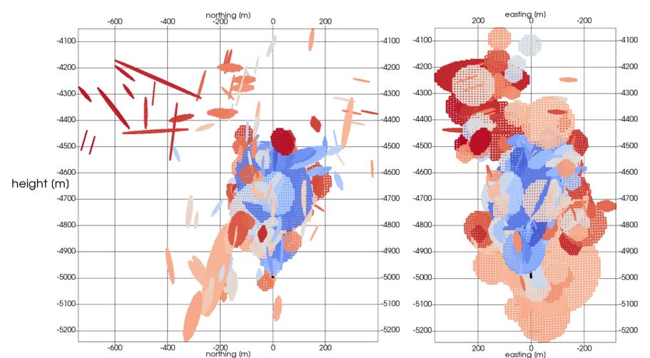
Figure 3: The network of discrete fractures derived from a forward simulation with the hybrid model is presented above, Note that the bottom of the well is located at  $(0, 0, -5.km)^T$ .
