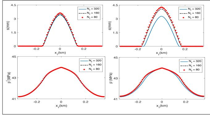
Further, the following figures depict how the failure propagation and the  $L_1$ -error evolves for slip solutions using different relations between grid and time step size.
