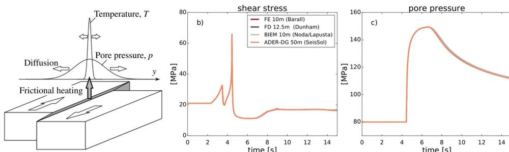
a) Sketch of the interplay of frictional heating and pore pressurization [7] b) Shear stress and c) pore pressure on one point of a 1D fault in a 2D domain (benchmark by the Southern California Earthquake Center). Note the excellent agreement of SeisSol with established Finite Element [9], Finite Difference [8] and Boundary Integral Methods [7].
