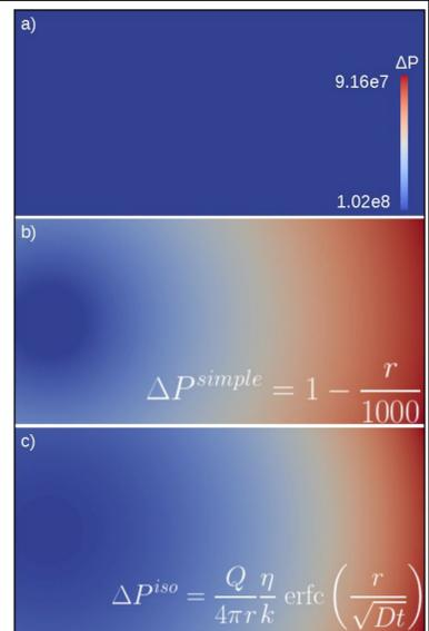
Different formulas to calculate pore pressure gradients. a) constant pore pressure, b) simple pore pressure gradient depending on nucleation size, and c) pore pressure solution in response to injection at a point source in an isotropic, 3D reservoir [3,4].
