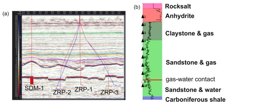
Fig.3. (a) Seismic section with monitoring wells. (b) Lithology of borehole SDM-1 and geophone locations (black triangles, geophone 9 was out of order).
