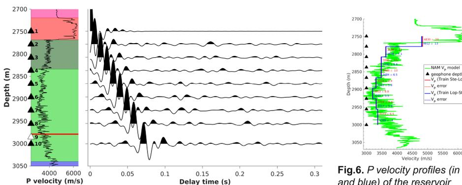
Fig.5. Stacked deconvolutions of train signals, using the signal of geophone 1 (~9000 trains, 03 Jul - 1 Dec 2015).
