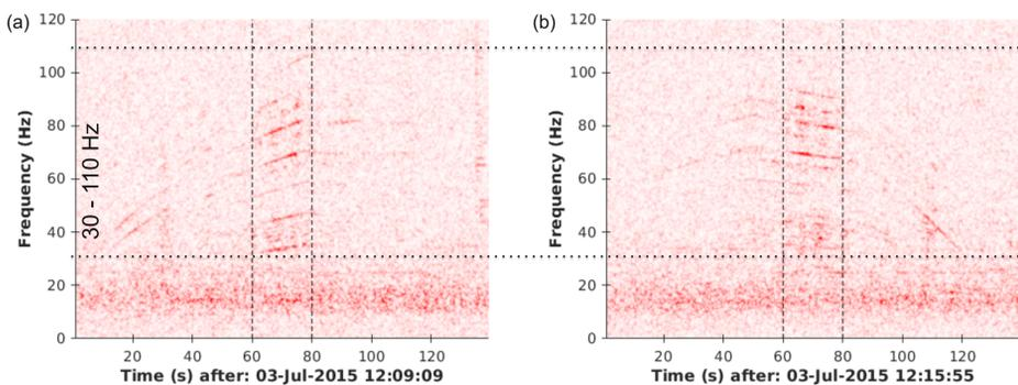
Fig.4. Spectrograms of train signals recorded by geophone 10. (a) A train departing from Stedum station (to Loppersum). (b) A train approaching Stedum station (from Loppersum).
