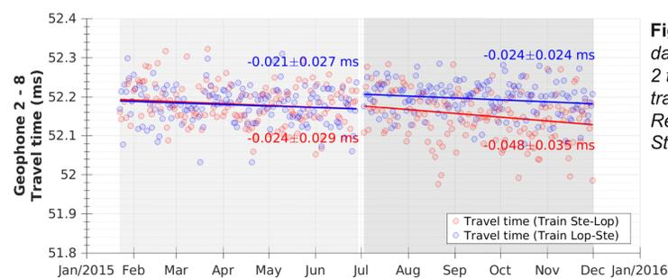
Fig.8. Travel times (from daily stacks) from geophone 2 to 8 with linear fit. Blue: trains Stedum → Loppersum; Red: trains Loppersum → Stedum.
