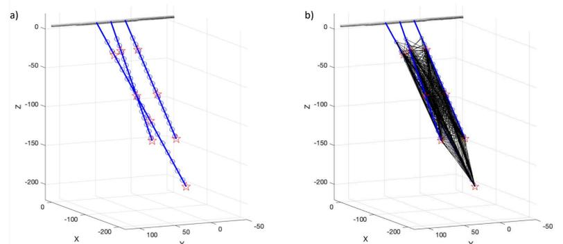
Figure 6: a) Geometry of source and receiver positions in the three wells and b) the resulting raytraces for all source-receiver combinations.
