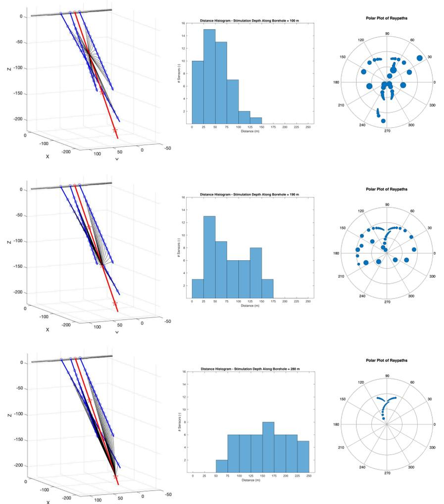
Figure 5: Ray-tracing for events at different locations along the stimulation well and the network of seismic sensors in three surrounding monitoring boreholes (left) together with the histograms of sensor distances (center) and the polar-plot of the individual seismic rays (right). Size of the circles corresponds to the source-receiver distance.
