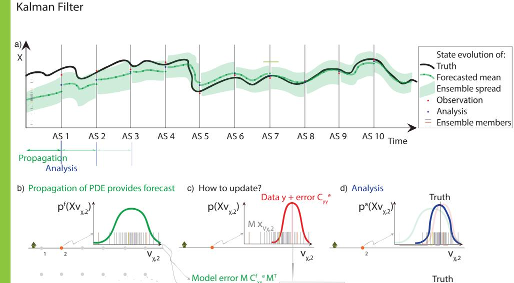
Fig. 2: **Cartoon explaining Ensemble Kalman Filters** in a) time, highlighting how ensembles a) forecast the prior, b) relate to the data, and d) form the analysis.
