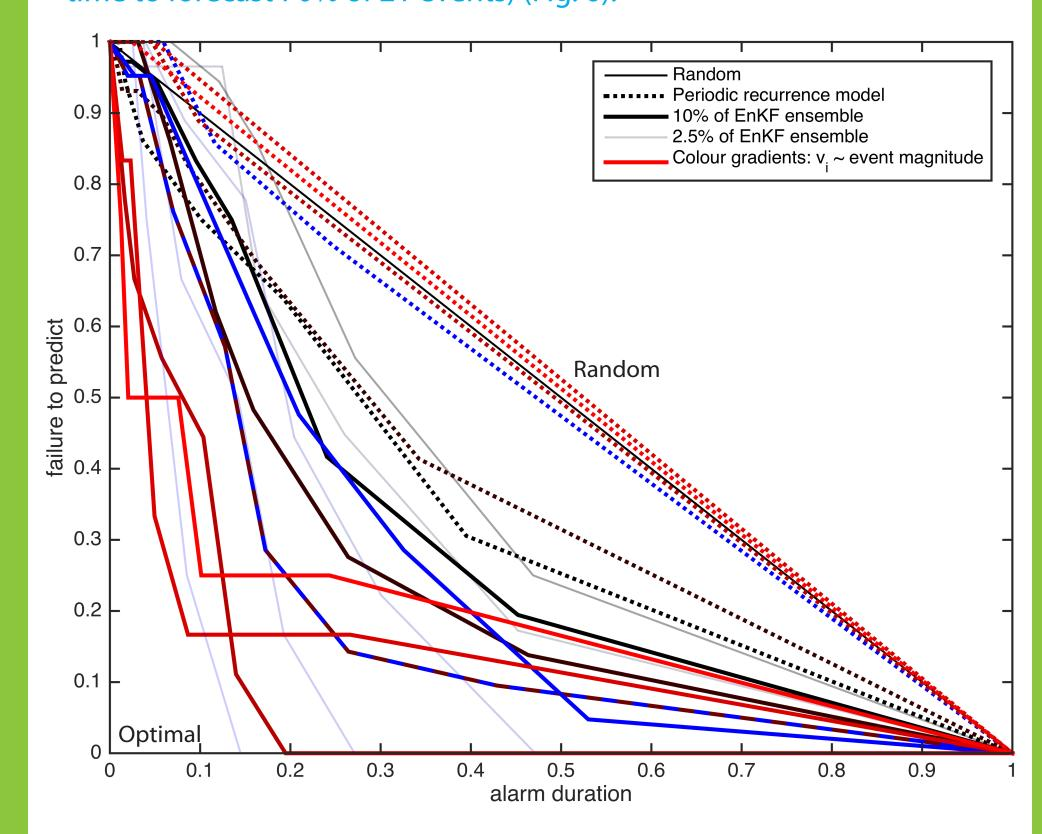
Fig. 6: Error diagram to assist decision making on earthquake forecasting. An alarm sounds when six different velocity thresholds (~event sizes) are passed (different lines). We use two different percentages of the assemble to sound an alarm (solid black to red, when increasing size, and transparent black to blue).
