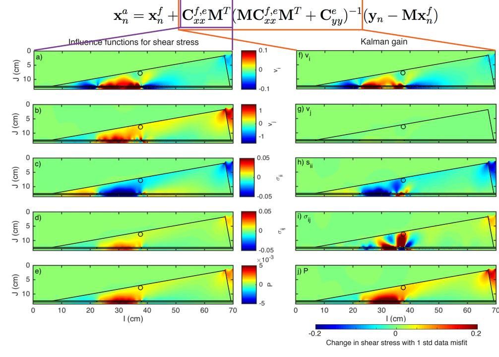
Fig. 9: **Information from physical model on how to update shear stress through space** a-e) transposed influence functions show how shear stress covaries with observations of each type f-j) scaled Kalman gain shows how to update shear stress due to a 1 std data misfit of each data type
