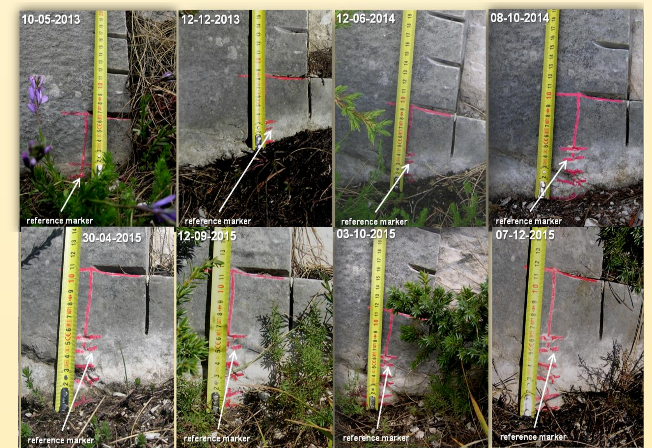
Measurements of bedrock scarp exposure through the relative position of the FSEC at the time of each measurement (Kastelic et al., 2017)
