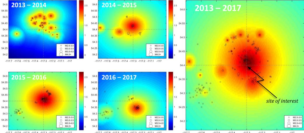
Maximum observed ground motion each year (from catalogue, with random draw of PSA from ground-motion distribution). Maximum moves each year, and area of maximum motion fills over time.
