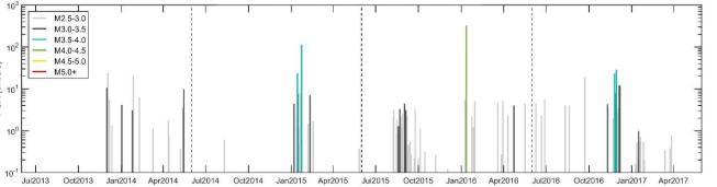
By comparing ground motion parameters at a site as obtained from the actual catalogues with corresponding random samples from the simulated catalogues, we demonstrate the effect of clustering of motions in time on hazard. Temporal distributions are different but overall hazard is reproduced.
