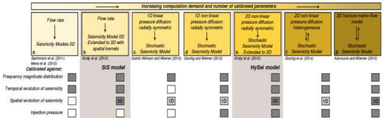
**Figure 29:** Evolution of induced seismicity models that are potential candidates for an Advanced Traffic Light System in geothermal projects (from Király et al., 2015)
