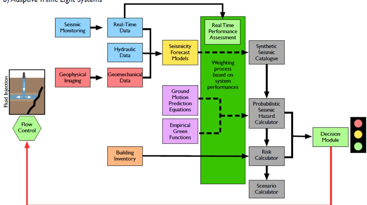
**Figure 31:** a) Classical Traffic Light System. Decisions are based on observed magnitudes and ground motions. Thresholds are defined in a static manner taking geotechnical information into account to the extent possible. b) Proposed Advanced Traffic Light System. Decisions are based on a forward looking, probabilistic and adaptive framework. Models are assessed in near real time and weighted accordingly. After Grigoli et al. (2017).
