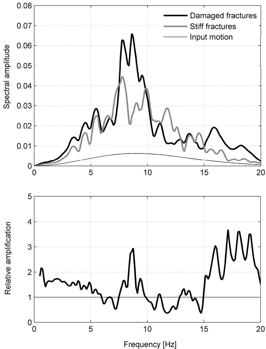
**Figure 5:** a) Spectra of Ricker wavelet input motion, slope response with uniformly stiff fractures, and response of incipient instability including selectively reduced-stiffness fractures resulting from damage (see Fig. 4b). b) Ratio of damaged slope spectra to that from the simulation using uniformly stiff fractures, showing relative spectral amplification.
