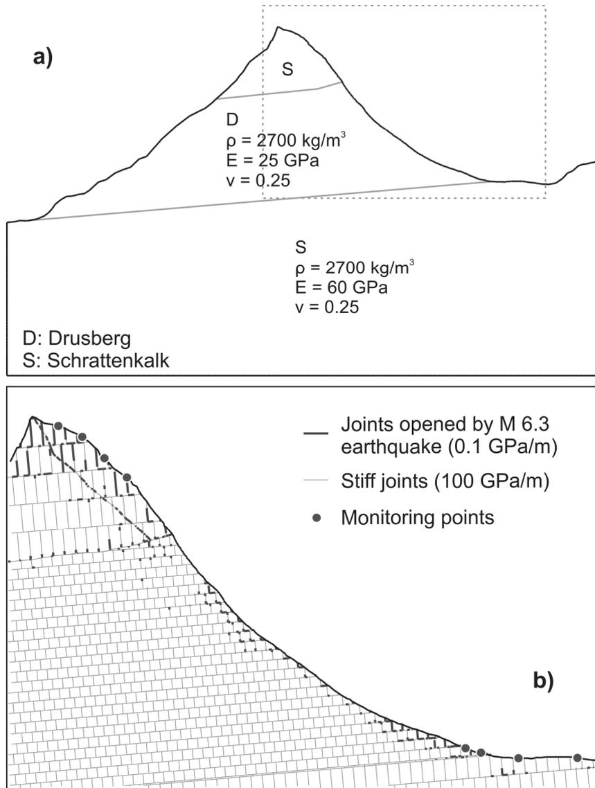
**Figure 4:** a) Geometry and select properties of the Rawilhorn model implemented in UDEC. b) Detail of the instability area showing open joints after the earthquake simulation, and their corresponding new lower assigned stiffness.
