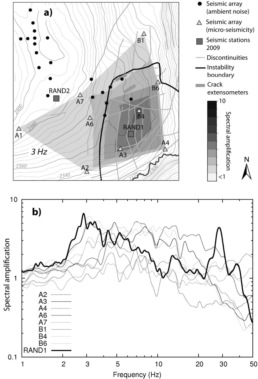
**Figure 2:** a) Layout of measurements at Randa shown together with key discontinuities and the instability boundary. SRSR calculated from earthquake recordings are shown resolved at 3 Hz and an azimuth of 135°. b) Mean SRSR for all stations as a function of frequency. Modified from Moore et al. (2011).
