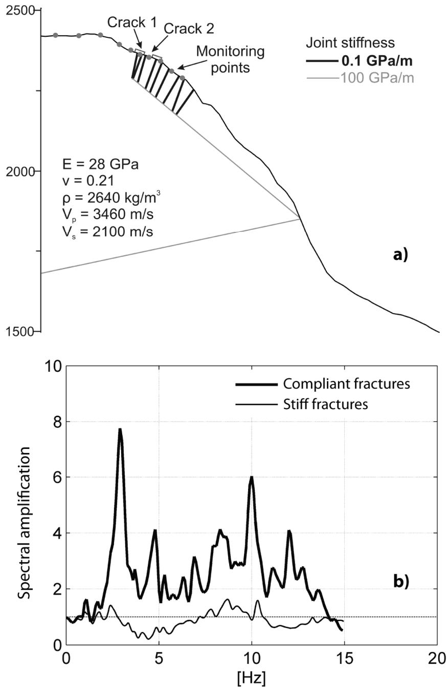
**Figure 3:** a) Simplified model of the Randa instability implemented in UDEC. b) Modeled spectral amplification comparing stations within and outside the instability and assuming compliant or stiff fractures. Modified from Moore et al. (2011).
