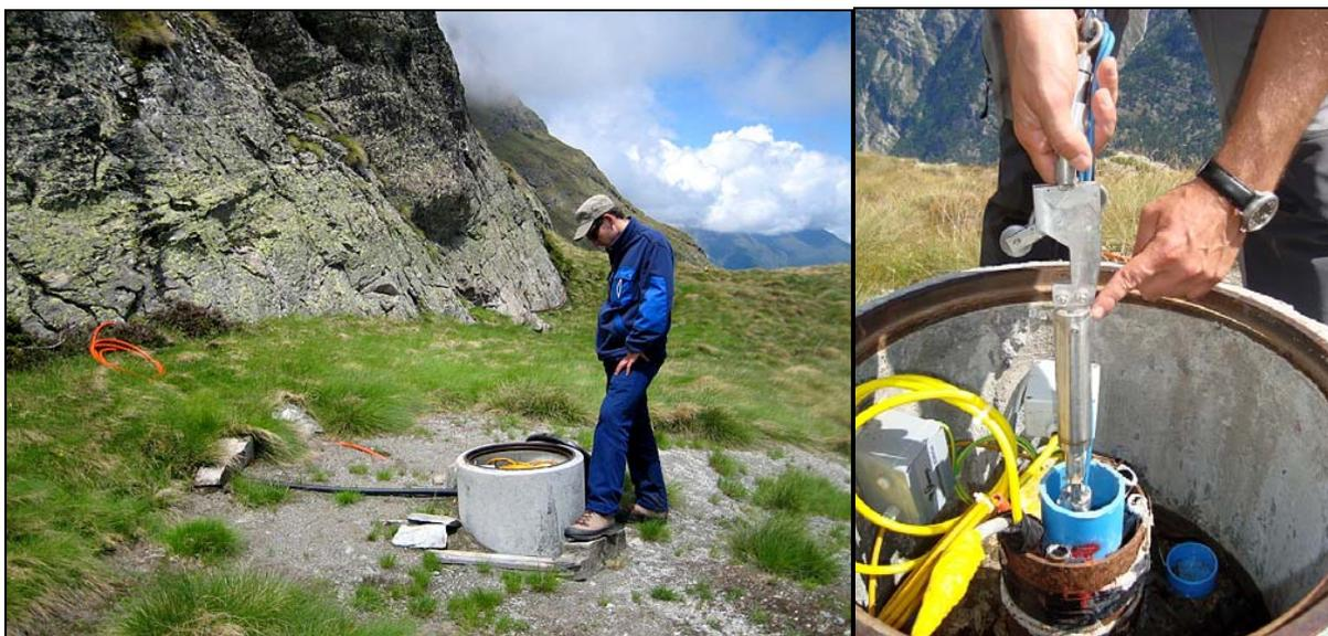
**Figure 8:** Borehole sb120 at Randa, showing the surrounding area and borehole top, and detail of the inclinometer casing and in-place inclinometer instrument.
