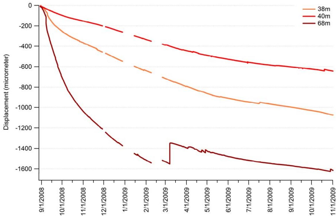
**Figure 3:** Deformation time series measurements from the three sensors at different monitoring intervals in borehole sb120 (data from just one sensor chain are shown). All sensors are shortening as expected. Accelerated shortening is seen immediately following sensor installation, which likely results from shrinkage of the grout. A number of transient steps and drops occur throughout the time history; one event from April 28, 2009 is highlighted in Figure 5. Dates are m/d/y.
