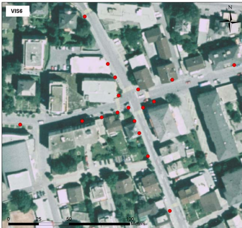
Figure 3.8.1: Sensor setup for array “VIS6” in Visp.
