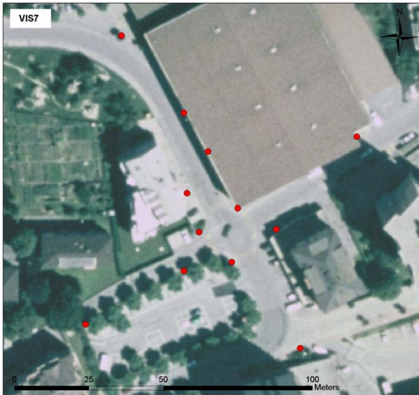
Figure 3.9.1: Sensor setup for array “VIS7” in Visp.
