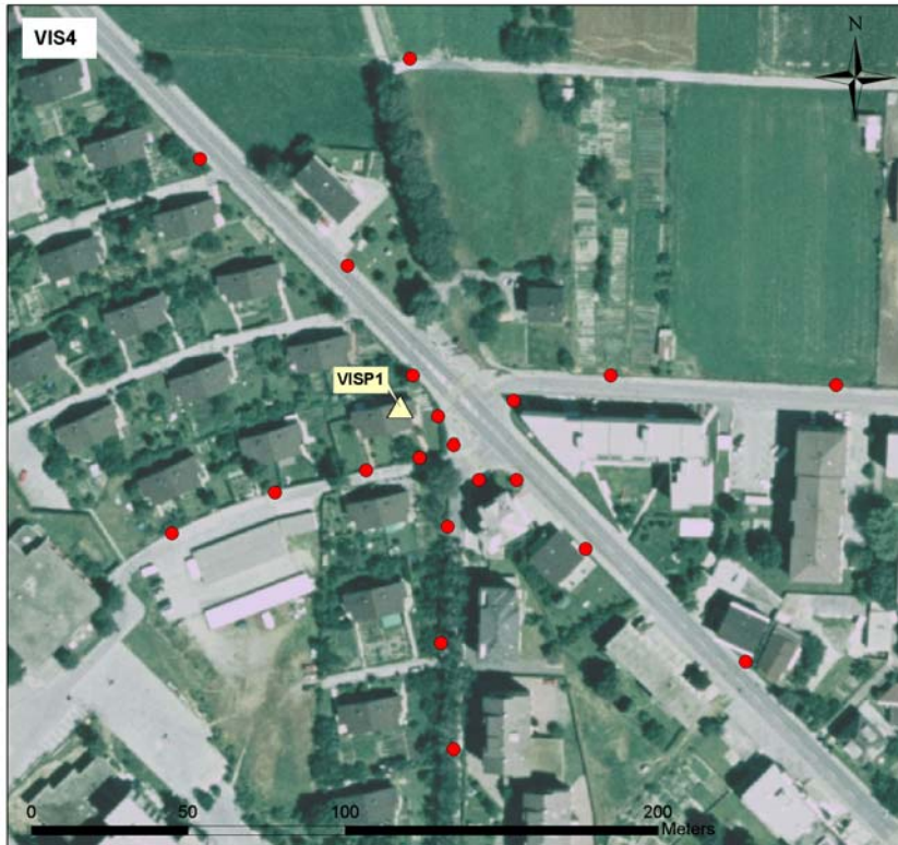
Figure 3.6.1: Sensor setup for array “VIS4” in Visp.
