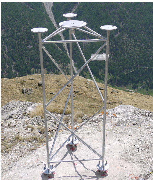
Figure 5: Mounted pillar with centered bolt (left) and antenna position adjusting perpendicular to the center bolt using a pillar base and an optical plummet (right)
