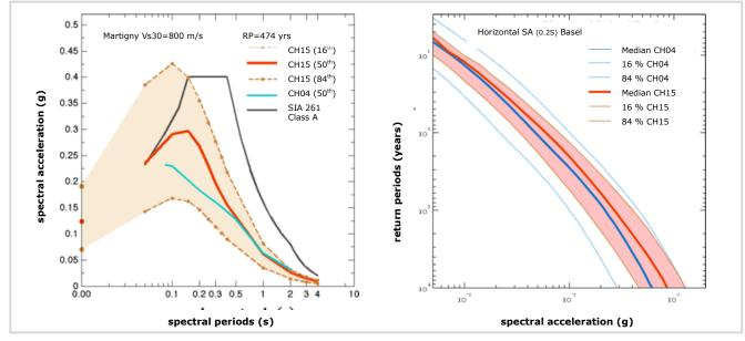
The figure on the **left** shows an example comparison, at Martigny, of the 2015 hazard model (CH15) with the 2004 model (CH04) for various frequencies and the SIA-defined standard spectra (SIA261).Compared with CH04, CH15 covers a wider frequency range and for certain frequencies shows somewhat higher hazard. On the **right** we compare the models using so-called hazard curves — the expected return periods of spectral acceleration — for Basel at a frequency of 5 Hz.
