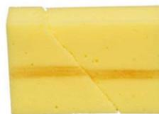
Figure 3 Reverse fault, before slip. BGS ©UKRI
