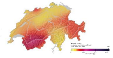
Horizontal acceleration at 5 hertz; the probability of a building constructed on rocky subsoil (reference rock) experiencing this is 10 % within fifty years.
