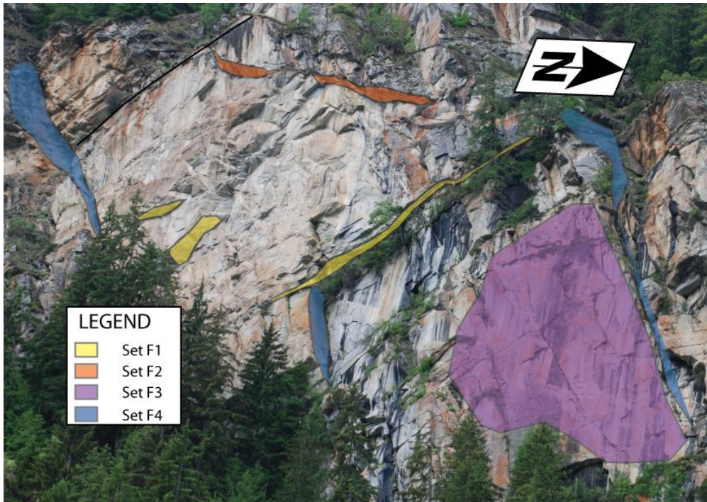
Figure 2.21. Photograph taken in the area of Saenggini close to the Blattbach River showing the four main large scale fracture sets for the study area.
